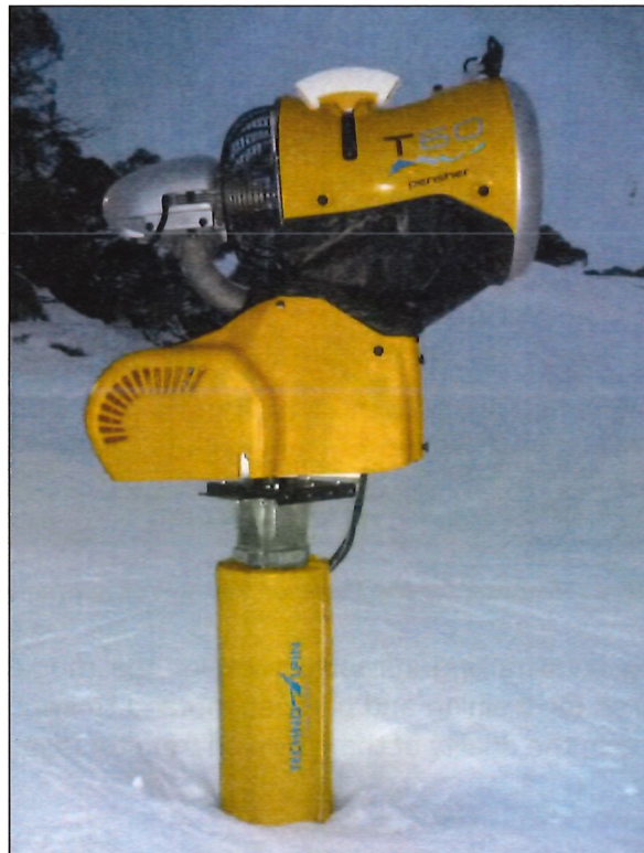
Figure 8: Typical fan gun to be used
